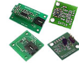
Temperature and Humidity Sensors
